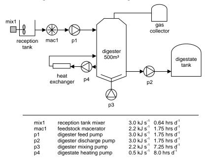
Figure 2: electricity requirement for a simplified digester system
