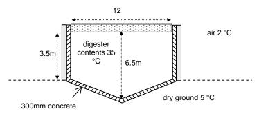
Figure 3: a simple digester structure used in calculation of energy loss.
