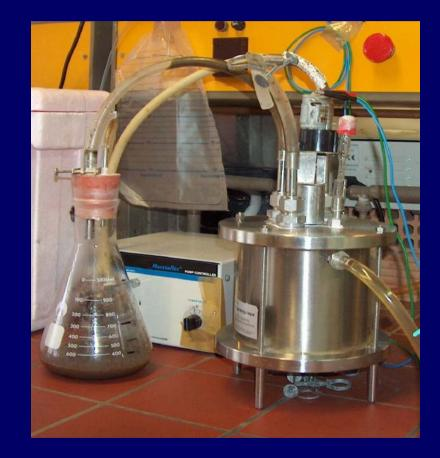
Active volume: 500 mlOperating conditionsTemperature35 or 55 °CHRT (h)14 - 30Flow rates (ml/d)300 - 1600Loading rates<br/>(g TS/d)20 - 90
