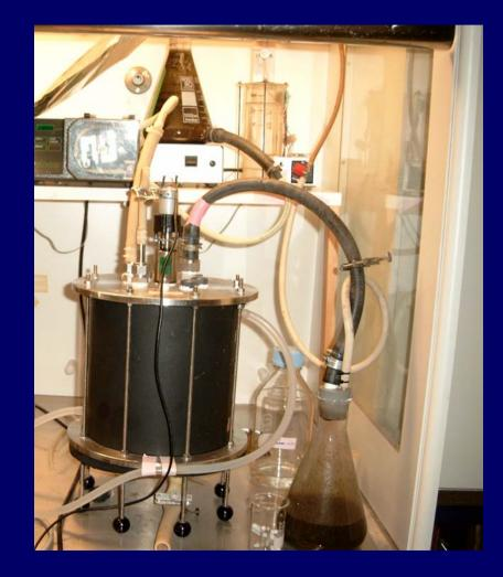
Active volume: 3 L **Operating conditions** Temperature 35 or 55°C HRT 20 d Flow rate 150 ml/d Loading rate 7 g TS/d
