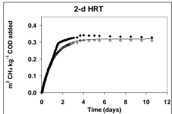
Fig. 2d. Methane production ( $m^3 kg^{-1} COD$  added) for liquor from a reactor with a 2.0 day HRT
