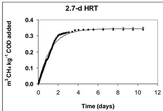
Fig. 2c. Methane production ( $m^3 kg^{-1} COD$  added) for liquor from a reactor with a 2.7 day HRT
