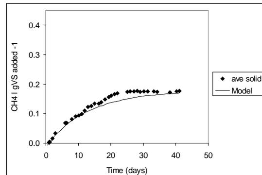
*Fig. 3b Methane production ( $\text{l gVS}^{-1}$  added) for separated solids from 4-day HRT*
