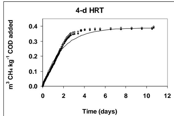
Fig. 2b. Methane production ( $m^3 kg^{-1} COD$  added) for liquor from a reactor with a 4 day HRT
