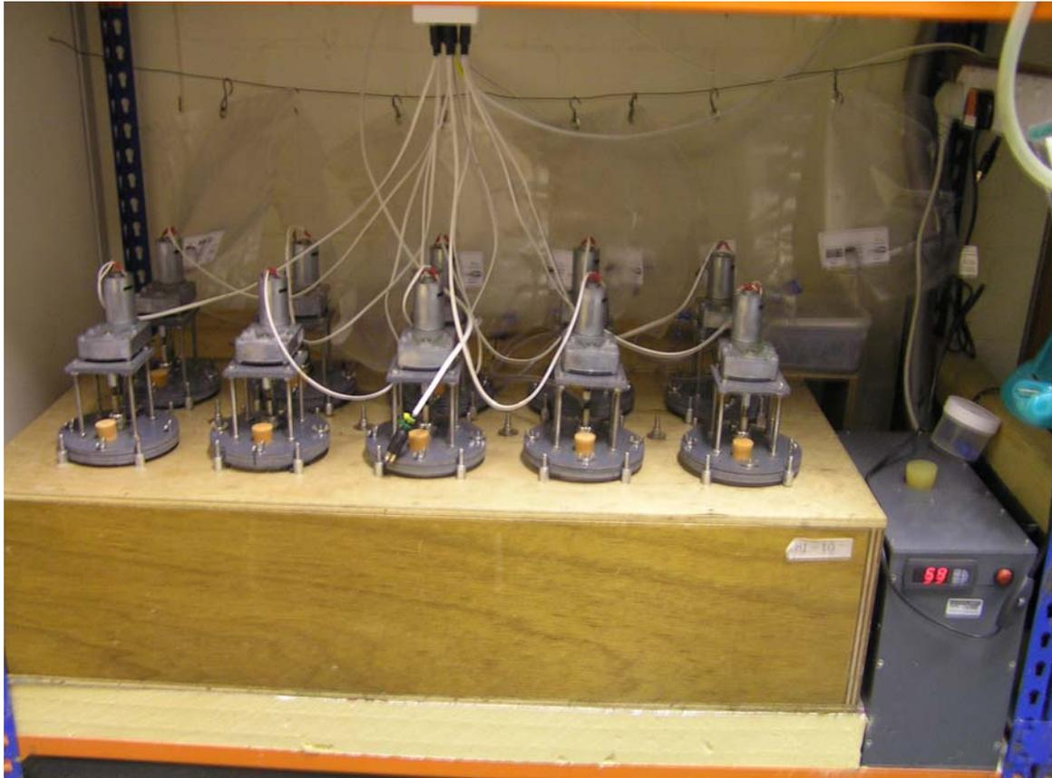
**Plate 1.** 1.5 litre working volume CSTR design digesters with gas sampling bags for biogas collection
