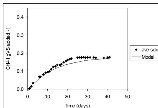
*Fig. 3b Methane production ( $\text{l gVS}^{-1}$  added) for separated solids from 4-day HRT*
