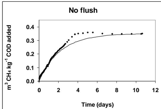
Fig. 2a. Methane production ( $m^3 kg^{-1} COD$  added) for liquor from a reactor with no flush
