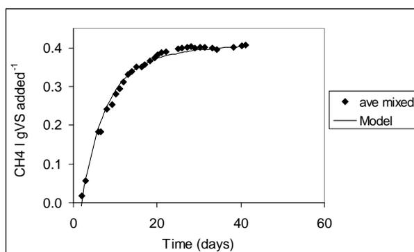
*Fig. 3a Methane production ( $\text{l gVS}^{-1}$  added) for mixed reactor contents from 4-day HRT*
