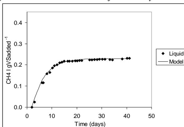
*Fig. 3c Assumed methane production ( $\text{l gVS}^{-1}$  added) for liquid fraction from 4-day HRT*
