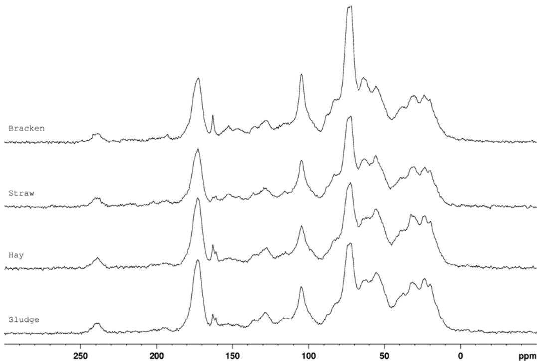
Figure 3.  $^{13}\text{C}$  CPMAS NMR spectra of bracken, straw, hay and sludge (maize) after anaerobic digestion.
