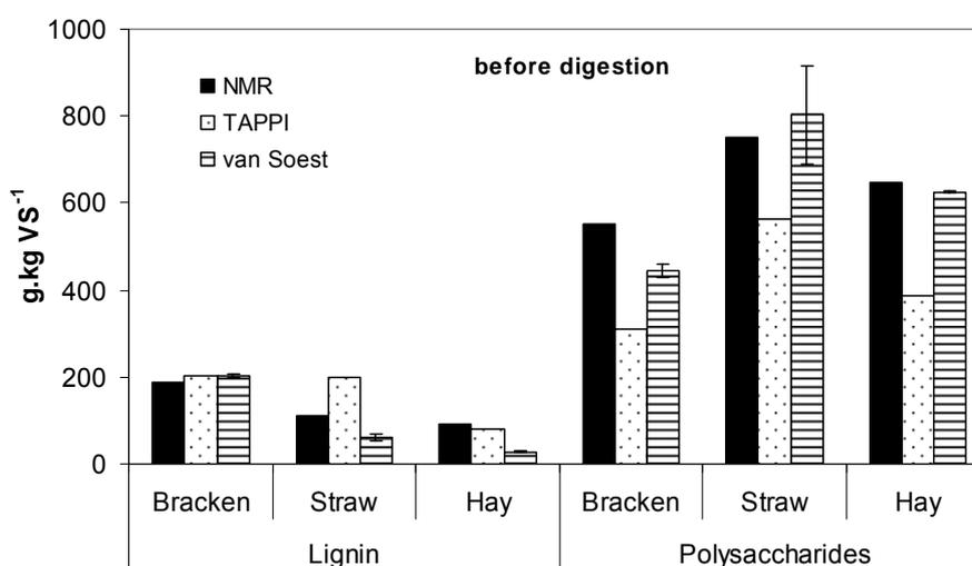
**Figure 4.** Lignin and polysaccharide concentrations of bracken, straw and hay obtained with <sup>13</sup>C CPMAS NMR, TAPPI and van Soest before anaerobic digestion.
