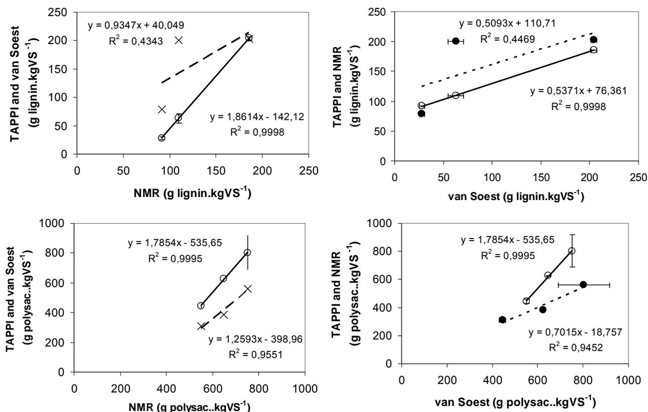
Figure 5. Correlation between lignin and polysaccharide methods before anaerobic digestion for bracken, straw and hay. NMR with van Soest (o); NMR with TAPPI (●); van Soest with TAPPI (x).
