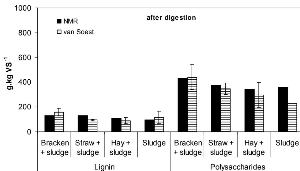
Figure 6. Lignin and polysaccharide concentrations of bracken, straw and hay obtained with <sup>13</sup>C CPMAS NMR and van Soest after anaerobic digestion.
