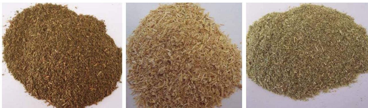
Figure 1. Ground and freeze dried bracken, straw and hay before anaerobic digestion.
