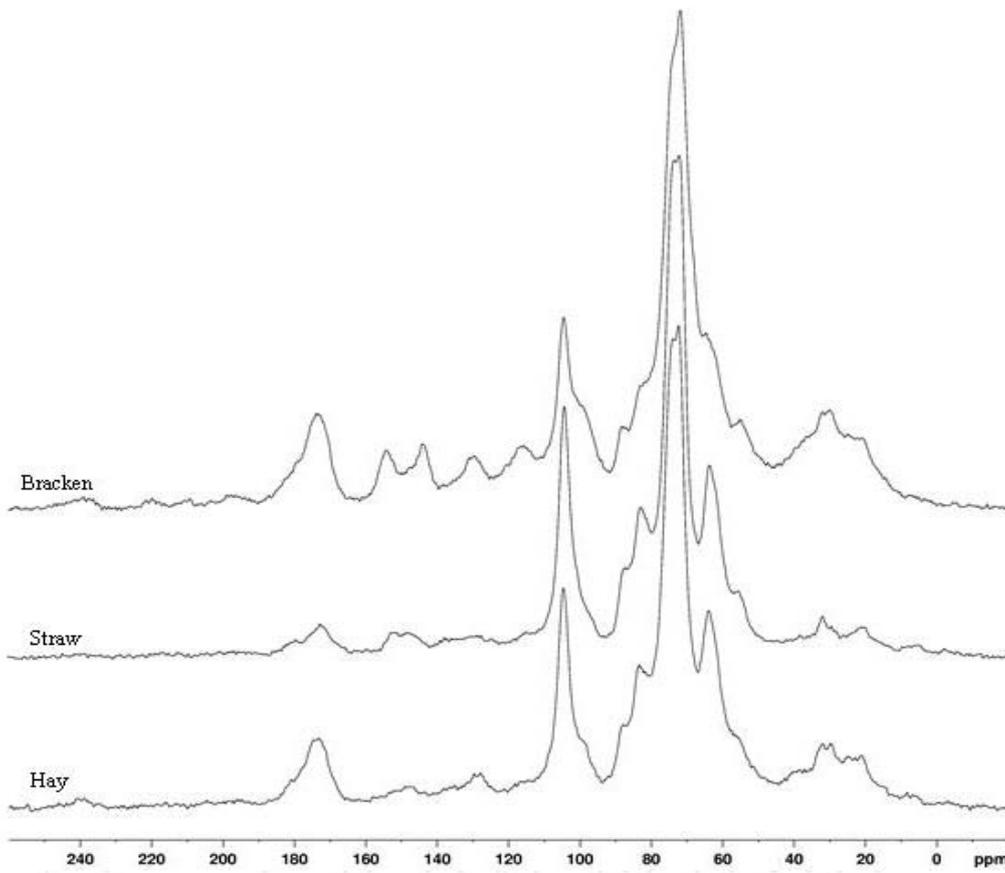
Figure 2.  $^{13}\text{C}$  CPMAS NMR spectra of bracken, straw and hay before anaerobic digestion.
