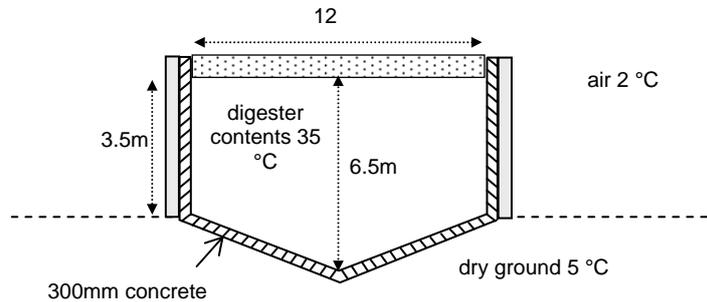
**Figure 3: a simple digester structure used in calculation of energy loss.**
