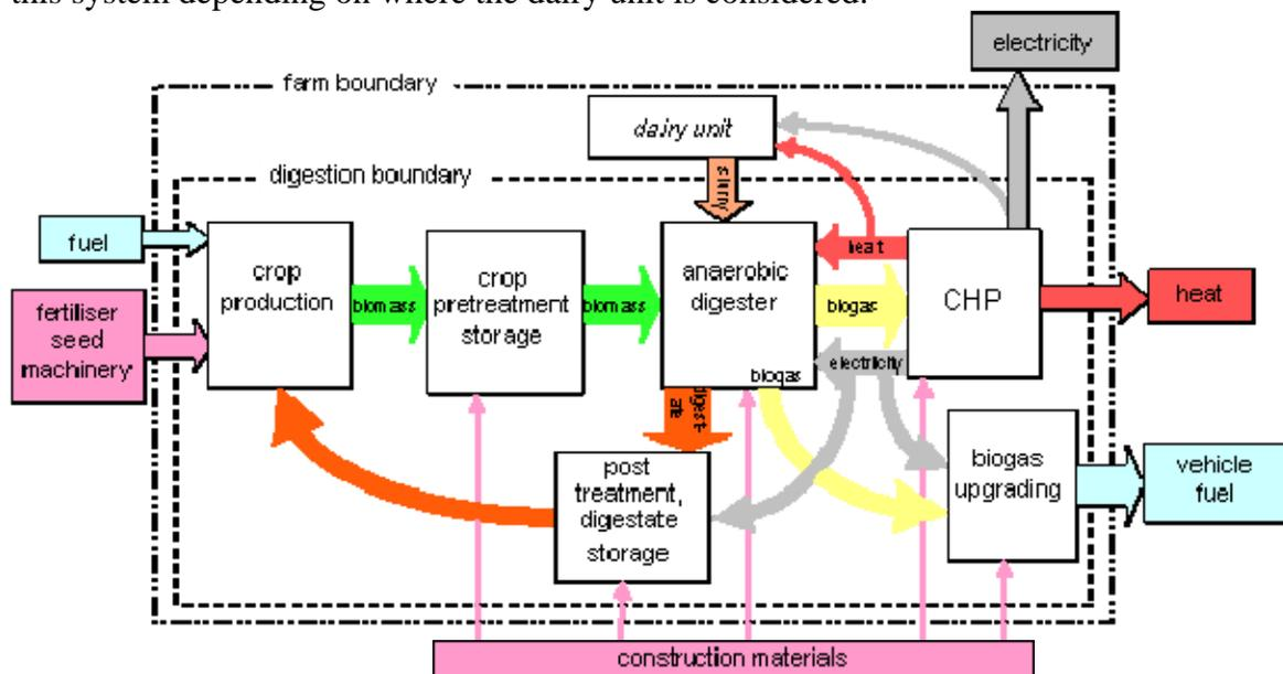
Figure 6: Boundaries for a mixed arable/livestock farm based digester
